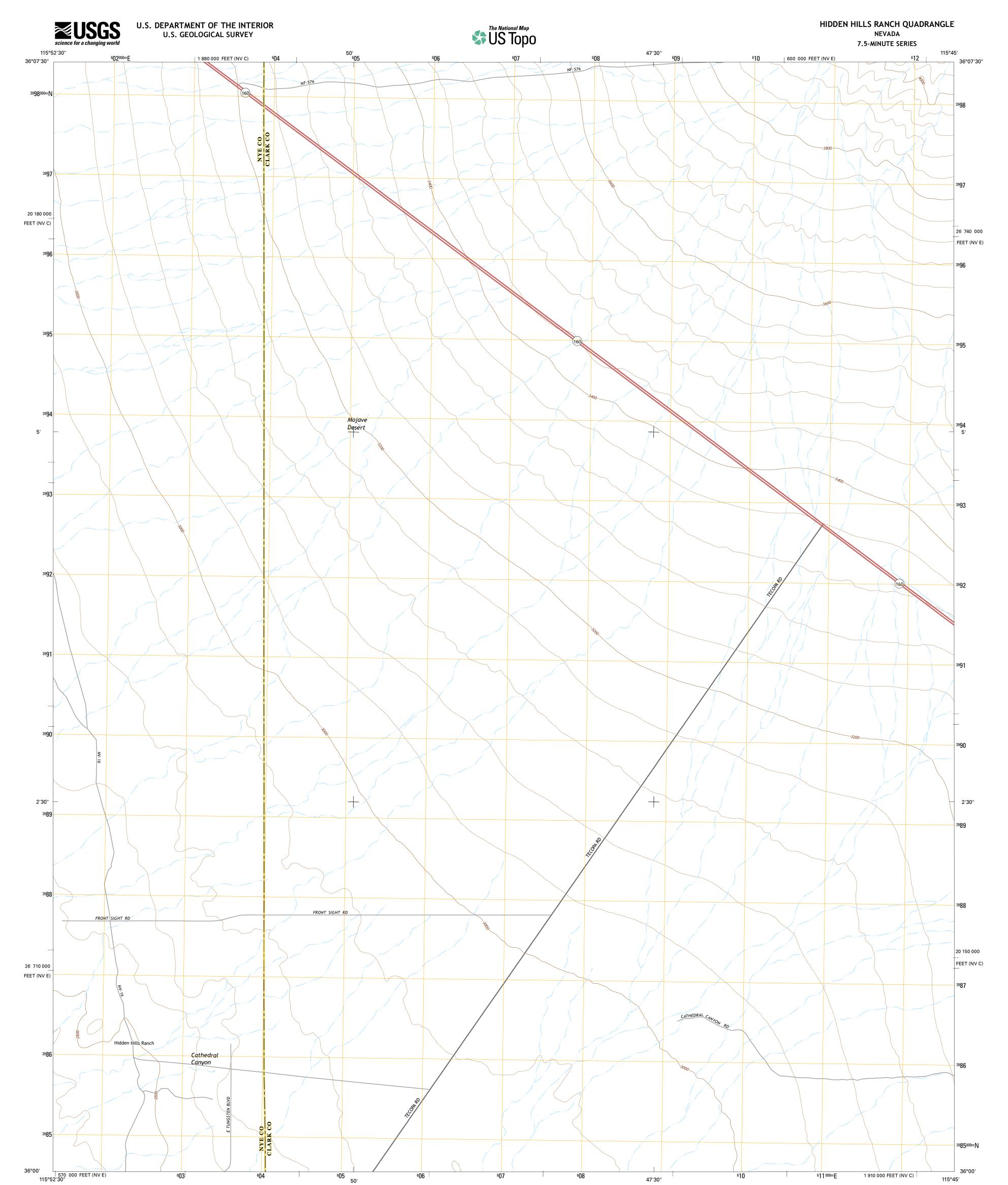
**Produced by the United States Geological Survey** North American Datum of 1983 (NAD83) World Geodetic System of 1984 (WGS84). Projection and 1 000-meter grid: Universal Transverse Mercator, Zone 11S 10 000-foot ticks: Nevada Coordinate System of 1983 (east and central zones)
