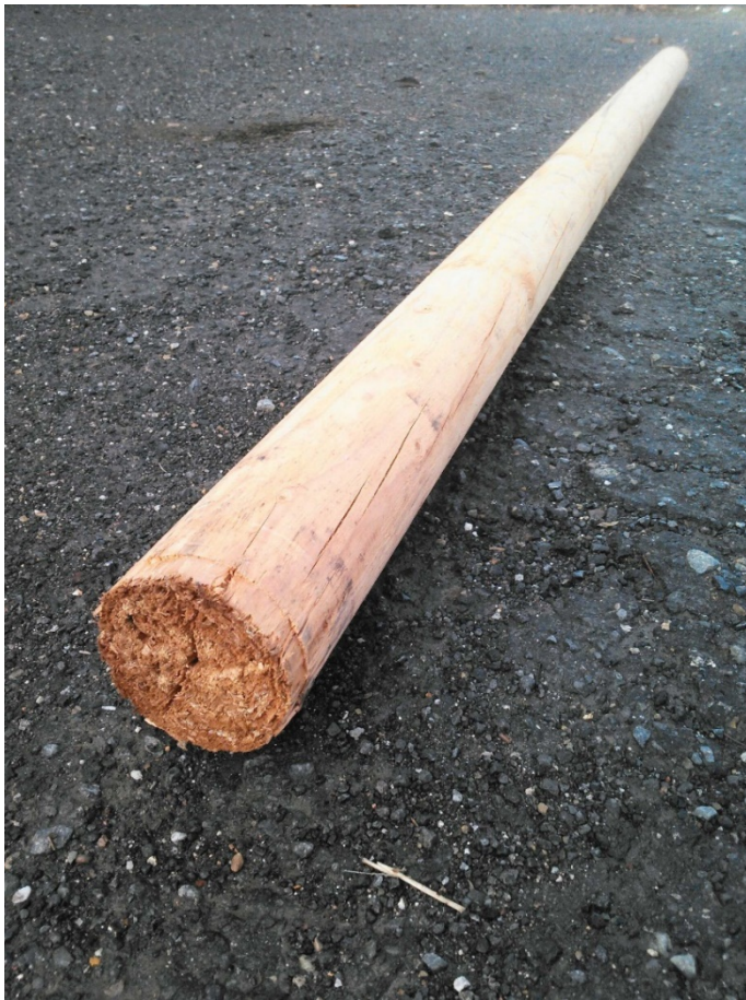
Figure 2 Example of 4" Doug Fir Peeler core. Use of this log type reduces variation and removes the step of peeling sample logs.
