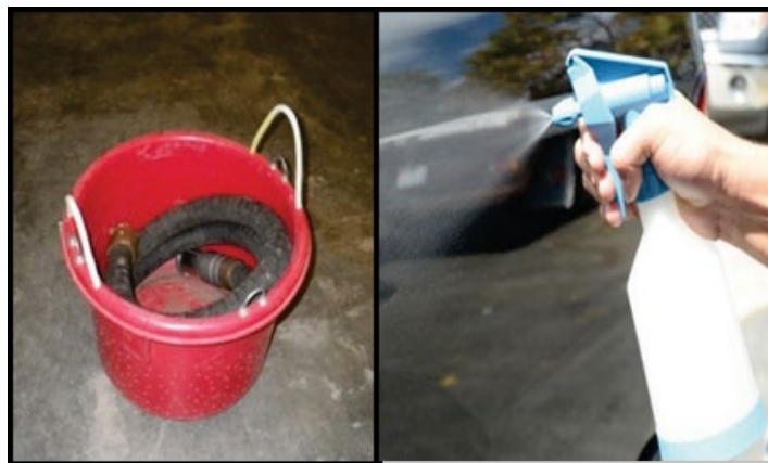
Figure 1. If drying or hot water are not options, draft hoses with foot valves can be decontaminated by submerging in a bucket filled with disinfectant.
