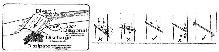
Watercourses: Work with READs to determine appropriate repair needs. Remove deposited soil from streams, watercourses, swales, or draws back to the original contour. Remove only as much as feasible without further damage to the watercourse. Restore bank channels at fire line crossings back to the shape seen adjacent to the crossing. Pull perched soil from drainage edges and spread it evenly across the fire line.
