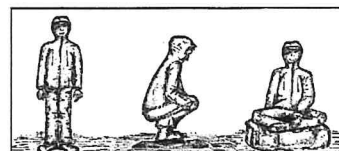
Fig. 4 Lightning positions: Put your feet together to significantly reduce the effects of ground current. If you have a foam pad to stand on or a pack to sit on, get on it. Crouch or sit to slightly reduce the effects of side flash and upward leaders.
