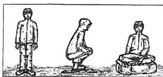
Fig. 4 Lightning positions: Put your feet together to significantly reduce the effects of ground current. If you have a foam pad to stand on or a pack to sit on, get on it. Crouch or sit to slightly reduce the effects of side flash and upward leaders.
