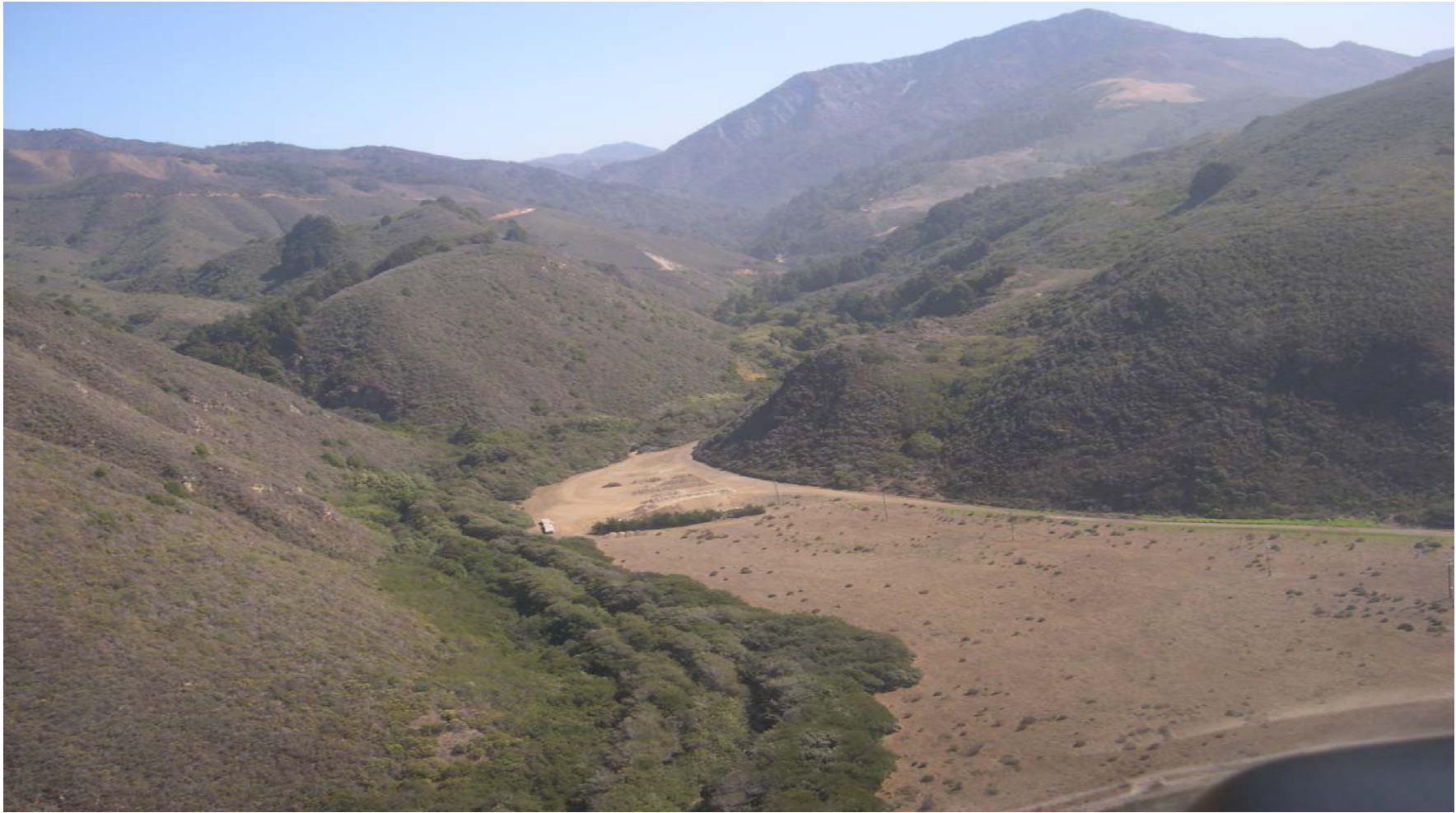
Figure 7: Lower Little Sur River valley just upstream of the Highway 1 Bridge from helicopter view. Wide valley above bridge is able to have flood water and debris settle on adjacent fill terrace. Valley at this point and upstream is wider and with a lower gradient with well developed stream side vegetation that should buffer high peak flows and allow the majority of floatable large wood and sediment to deposit and store over the valley reach. Threat of damage to Highway 1 Bridge over Little Sur River by large wood is unlikely.
