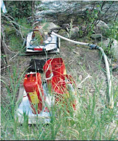
This setup had a 2-inch line running back to a hardened site that trucks could hook up to, fire up the pump, and fill >50 feet from the creek.
