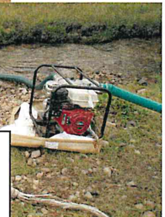
Improved bucket-screen on a trash pump to service 2 fold-a-tanks in a turnout up on the highway.
