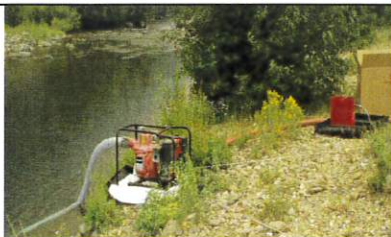
Trash pump servicing a pumpkin for tenders and engines.
