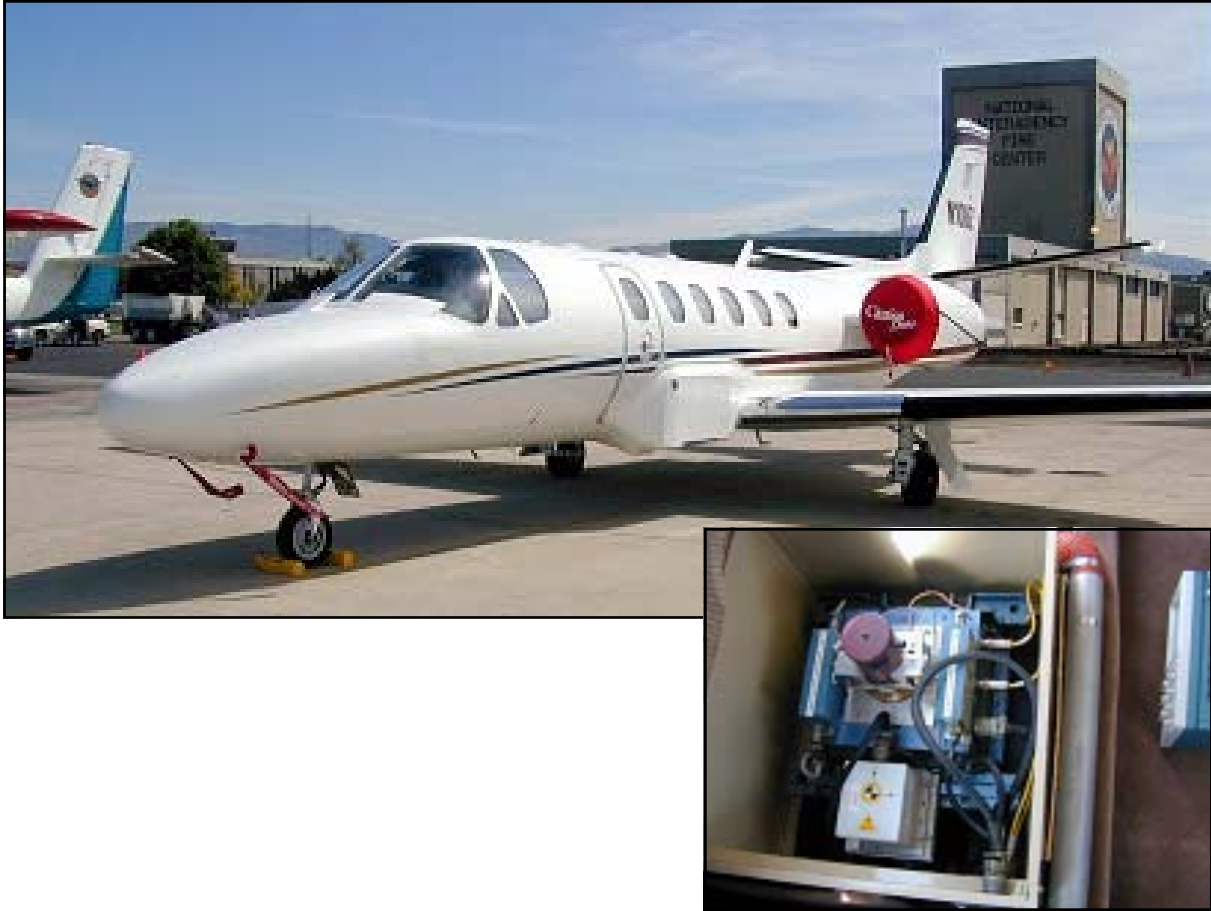
Figure 7—The NIFC Citation Bravo and the Phoenix line scanner, type 1 platform and sensor.
