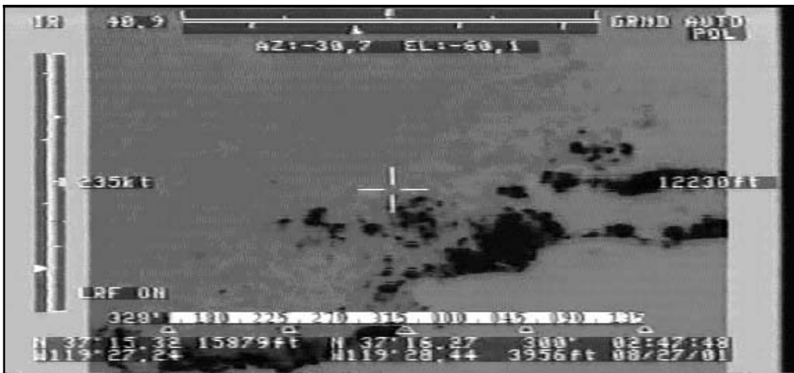
Figure 11—FLIR system display of a fire (black areas) source Nevada Air National Guard.
