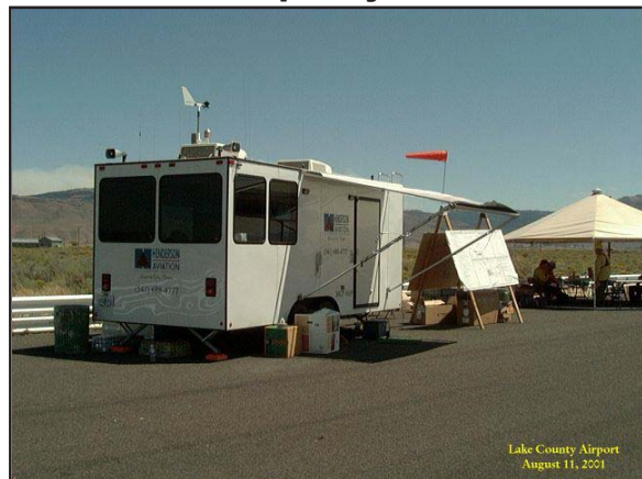
FIGURE 11-2 Example of a Trailer Rented for a Temporary Tower
