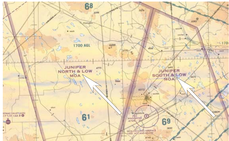
FIGURE 3-20 Example of a MOA on a Sectional
