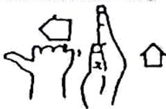
To indicate an APU disconnect at the end of the start sequence, one uses a fist with extended thumb (the hitchhiking signal) moving away from the raised, flat palm of the other hand. At night, pointing one wand and held vertically will be used for each respective signal.
