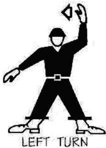
To turn the aircraft left, point to the left main landing gear wheel with the right arm and move the left hand as described above.
