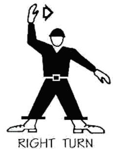
To turn the aircraft right, point to the right main landing gear wheel with the left arm and move the right arm as described above.
