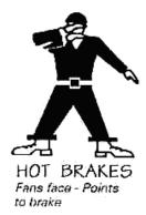
Occasionally quick stops on the runway and/or fast taxiing to the ramp result in hot brakes which are indicated by brake squeal, smoke from the main landing gear wheel assembly, or flames in the same area. The last two indications *dictate that this aircraft* not be moved into the pit if there is a possibility of the aircraft being disabled in the pit.
