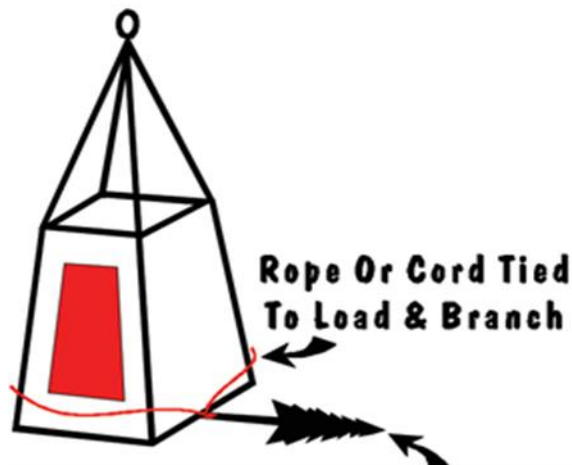
Exhibit 11.4 -- Rigging a Box-like Load with a Tree Branch as a Tail.
