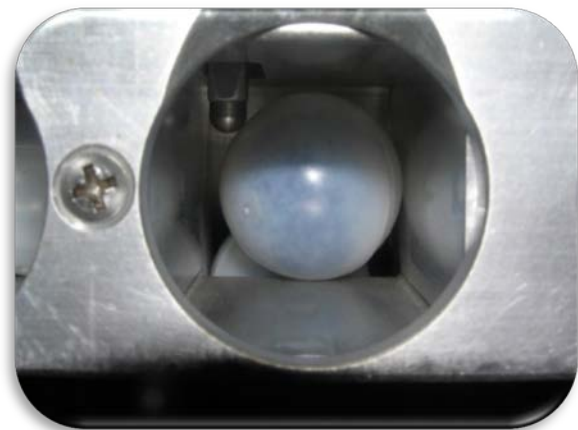
Figure 2. The shutoff finger in this chute does not make adequate contact with the Aerostat plastic sphere.
