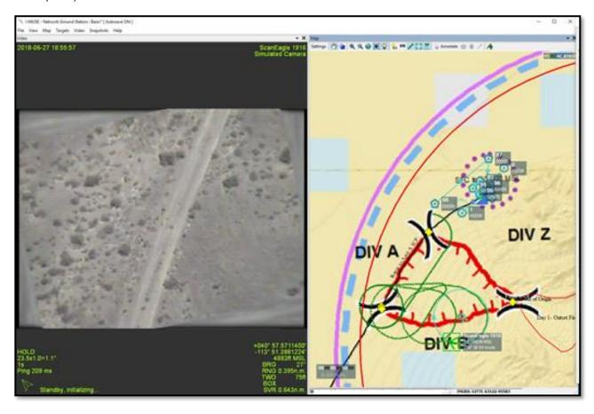
**Figure 2**: Screenshot of ground station display. Camera view is on the left and UAS location is on the right.
