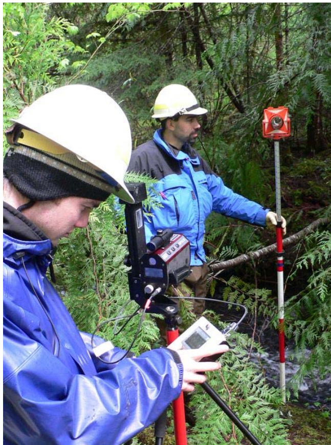
The watershed monitoring module uses laser levels to map the morphological characteristics of sampled stream sites. Photograph by Steve Lanigan
