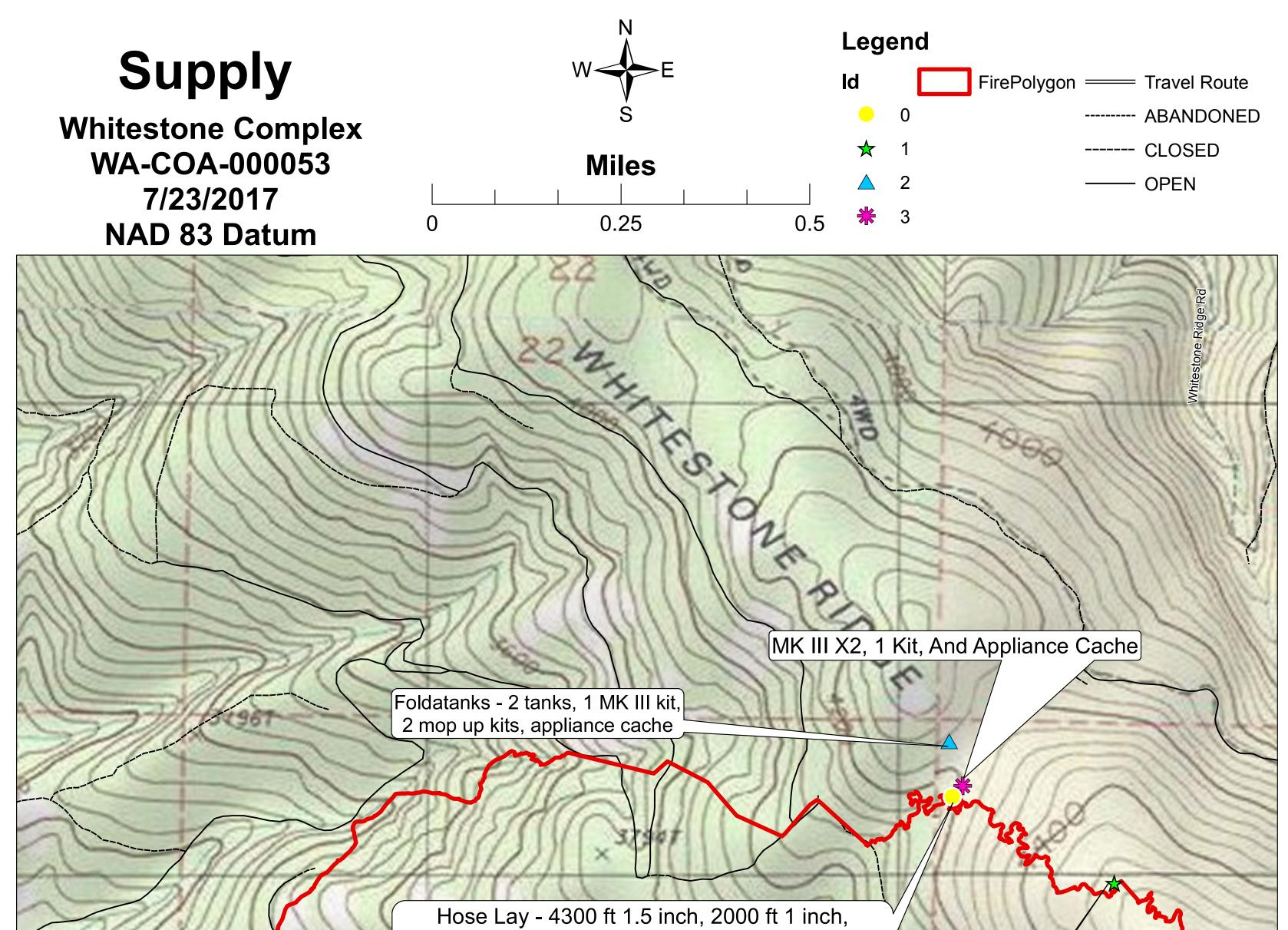
20 wyes reducers and nozzles. Also 500 ft of broken 1.5 inch, 1000 ft of spare 1.5 inch, and 900 ft of spare 1 inch
