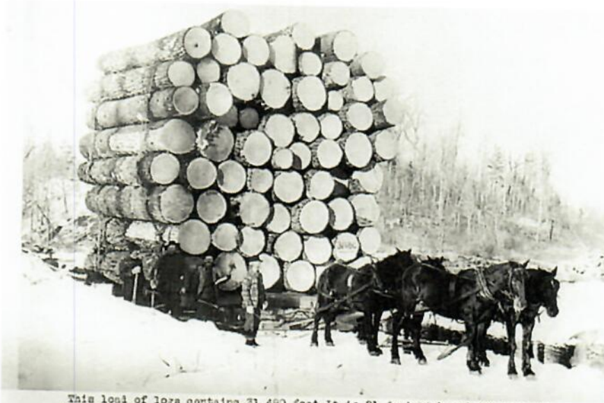
This load of logs contains 31,460 feet. It is 21 feet high and 20 feet wide. Hauled by four horses, one mile, by the Ann River Logging Co., on the 13th day of February, 1892. The size of the sled upon which this was hauled is as follows: The runners are 5 inches thick, 11 inches high, and 9 feet apart. The bars are 15x18 inches square, 12 feet long. The rooker is 15x18 inches square, 16 feet, 3 inches long. Estimated weight of sled and chains, 8 tons. S.C. Sargent, photographer, Taylors Falls, Minn.
