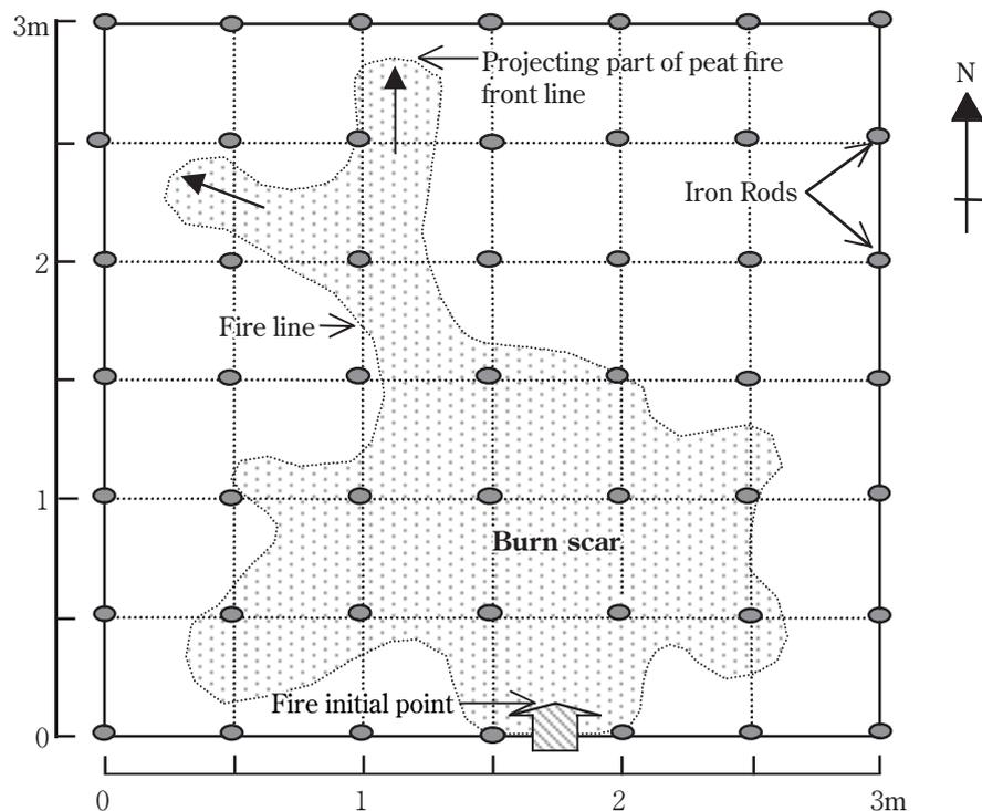
**Fig. 10.** A typical horizontal distribution of a burned surface peat layer with several projections of the fire front line at Plot-2 on August 10, 2002.
