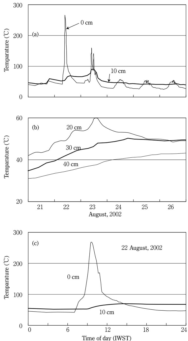
**Fig. 7.** The temperatures in peat layers during a fire event from August 21 to 26, 2002 in plot 3 of Kalamangan. (a) at ground surface and 10 cm depth from surface, (b) at 20, 30, 40 cm depth, (c) diurnal temperature changes of ground surface and 10 cm depth on the first day of the fire event, August 22, 2002.
