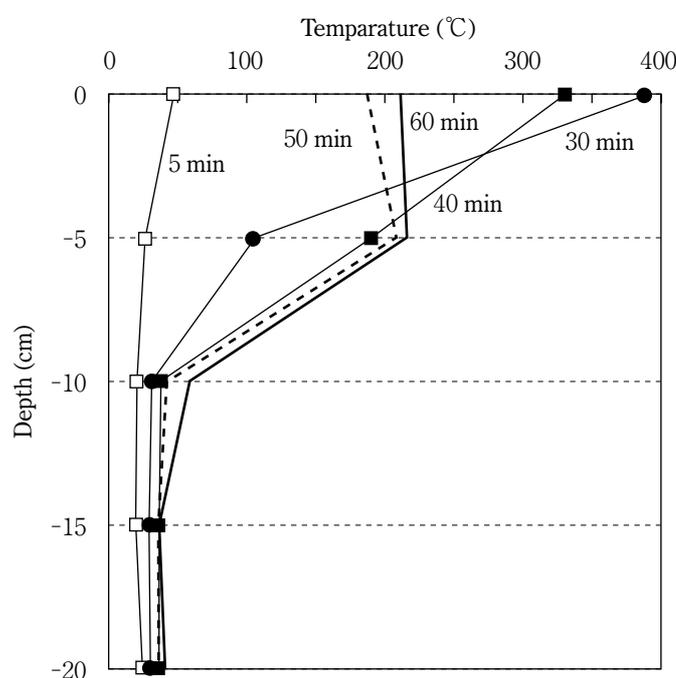
Fig. 8. Dry wood burning and pattern of temperature penetration into deeper peat layers on August 6, 2002 in Kalampangan.
