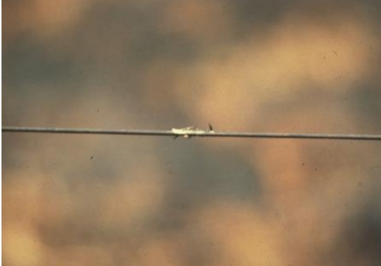
Figure 7.98. Grass residue is on the electric fence wire at the point of contact in this photo. Burn marks may also be present and may be the only sign of fence contact.
