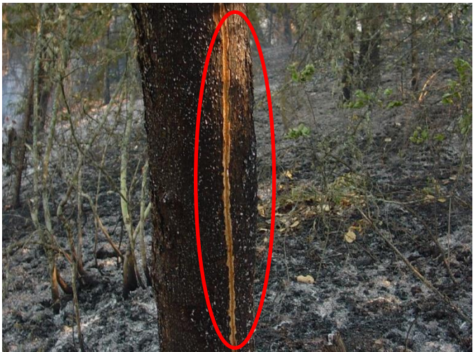
Figure 7.51. Electrical resistance scar on tree trunk.
