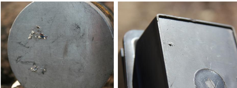
Figure 7.22. Friction particles found by using a magnet.
