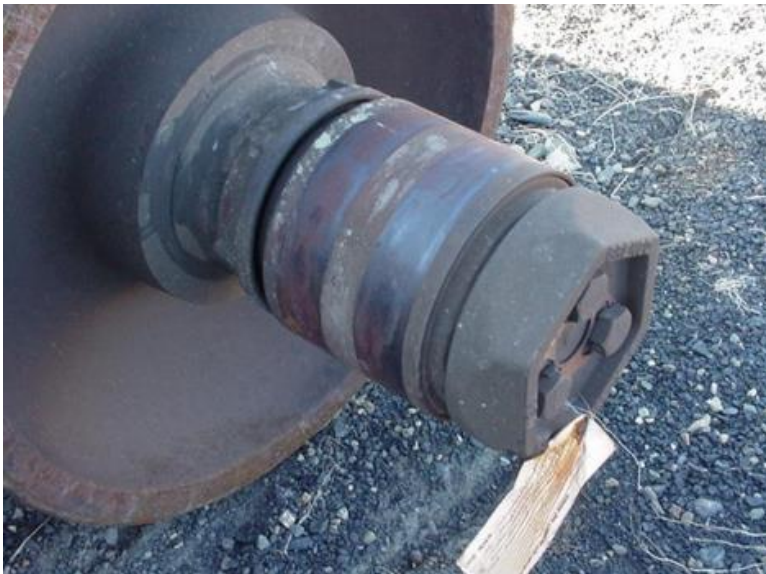
Figure 7.84. Roller bearing assembly that has been identified by a hotbox detector as being defective and tagged as "bad order"—a railroad term for a defective item or items.
