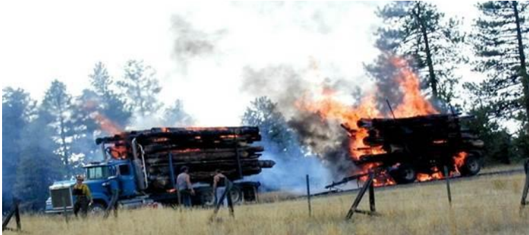
Figure 7.24. Log truck mechanical breakdown ignition factor.
