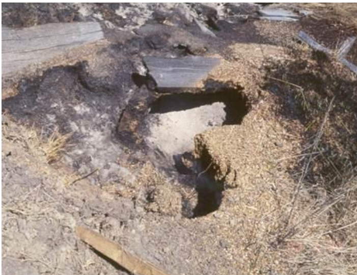
Figure 7.95. Typical spontaneous combustion fire effect in sawdust and wood chips.
