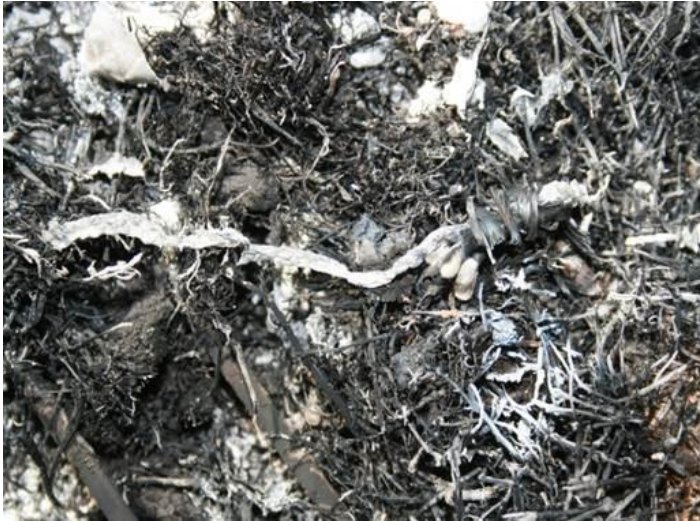
Figure 8.13. Cotton rope with matches tied to it prior to burning.
