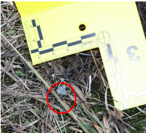
Figure 7.19. Catalytic converter particle.
