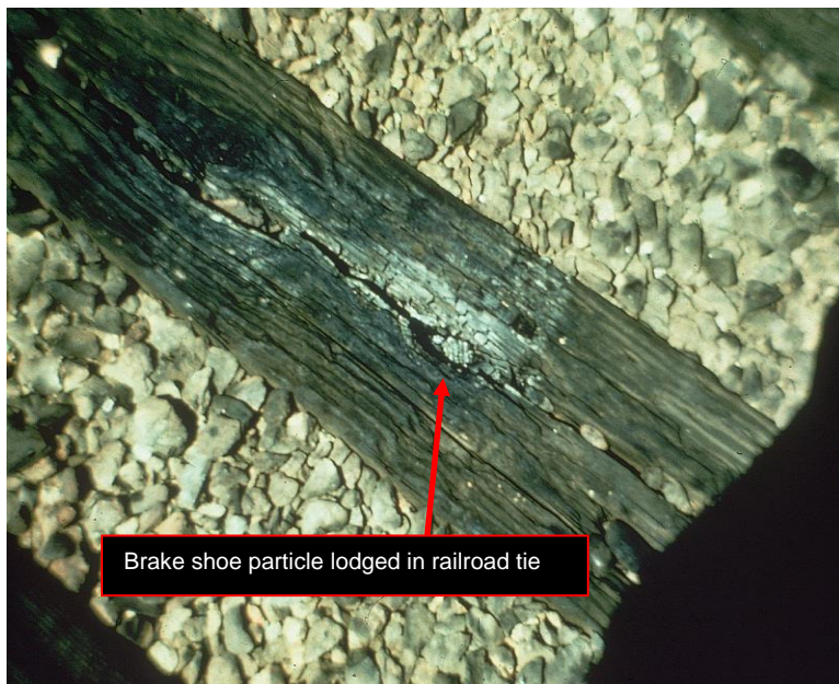
Figure 7.76. Brake shoe particle in railroad tie.
