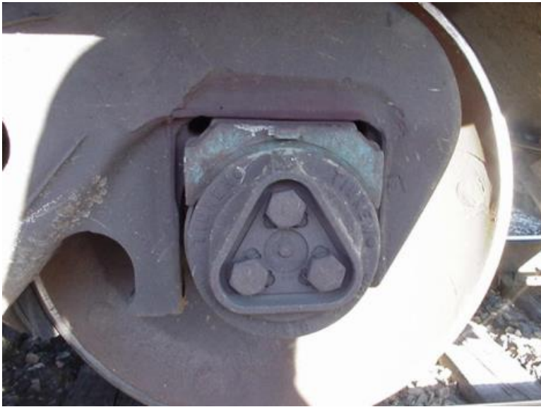
Figure 7.84. Roller bearing assembly that has been identified by a hotbox detector as being defective and tagged as "bad order"—a railroad term for a defective item or items.
