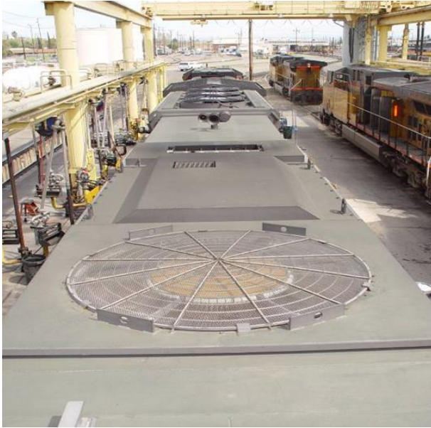
Figure 7.79. Dynamic brake grid exhaust outlet.
