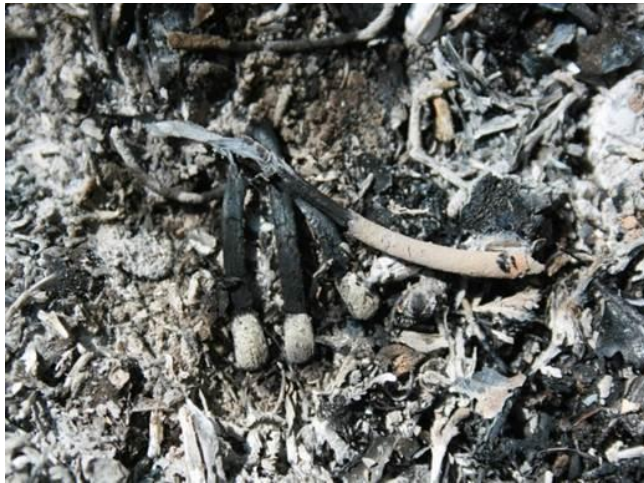
Figure 8.14. Burnt remains of incense stick with paper matches attached.
