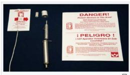
The M-44 consists of a capsule holder, a cyanide capsule, a spring-activated ejector, and a stake. Bilingual signs warn about the device.
